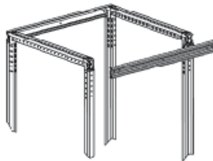
removable cross-member to simplify connection
