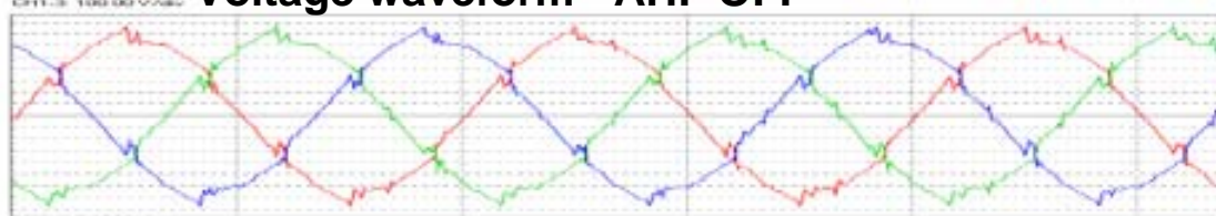
Voltage waveform - AHF ON
