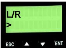
**Important Note:** In case of using Multifunction control Unit, you have the choice between “R” remote configuration mode or “L” local configuration mode (for more details see the training documentation or the User manual page 42)
